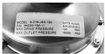
Typical label: "JBS" series rated to 16,000 psi
